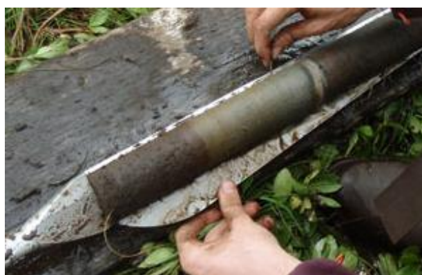
BELOW: Figure 3.1.2: A peat core collected using a Russian corer, containing a prominent white layer of volcanic ash.
